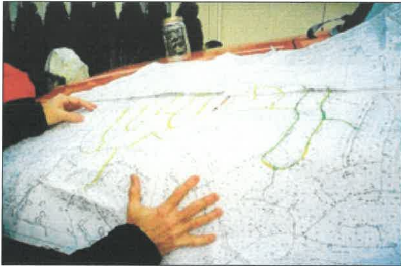
Distribution system maps can be used to identify flushing loops, valves to be opened or closed, locations of pump stations and hydrants, pressure-reducing valves, and other facilities.
