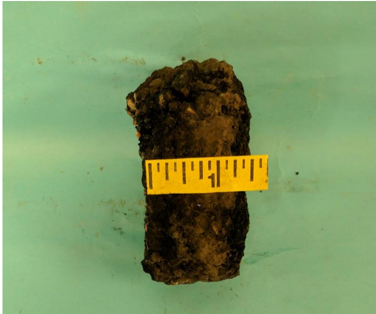
PHOTO 5: B-10 Recovered: 1.75" Field Thickness: 3.0"
