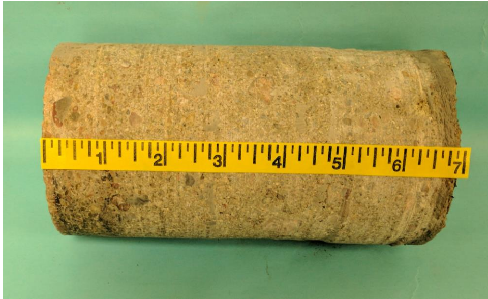
PHOTO 3: B-8 Recovered: 7.0" Field Thickness: 7.0"
