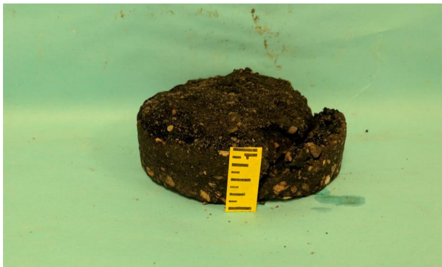
PHOTO 3: B-8 Recovered: 7.0" Field Thickness: 7.0"
