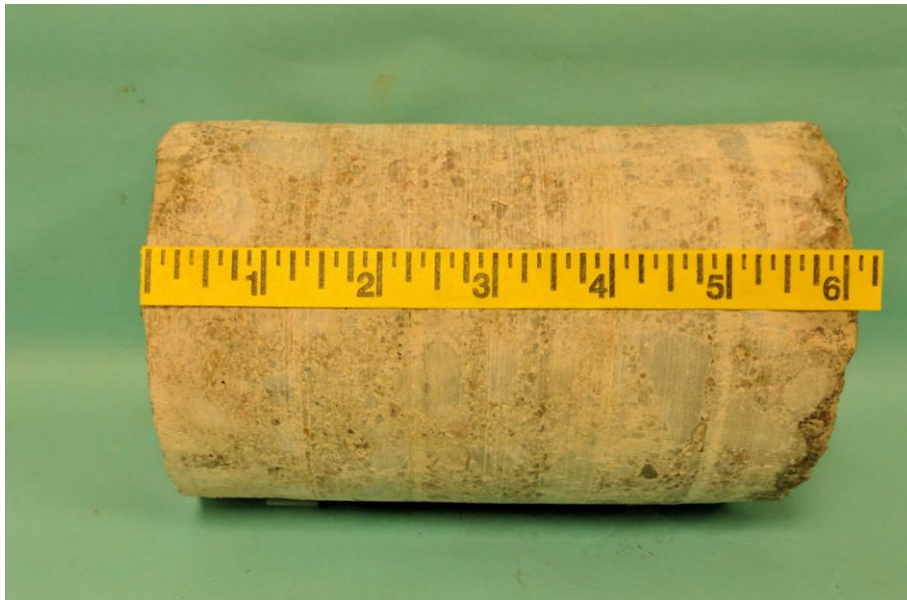
PHOTO 2: B-7 Recovered: 6.25" Field Thickness: 6.25"
