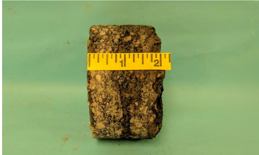
PHOTO 1: B-6 Recovered: 2.25" Field Thickness: 2.25"
